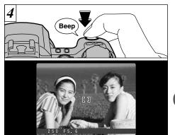
With the shutter button still held down halfway (AF/AE lock), move the camera back to the original image and press the shutter button down fully.
